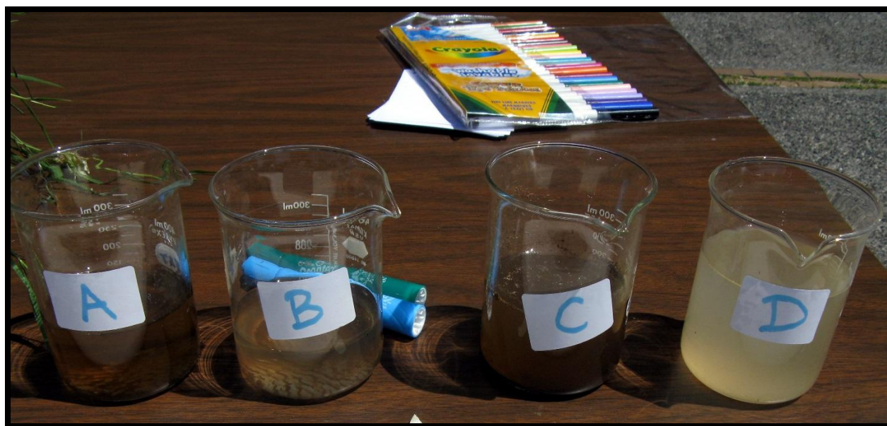
Figure 3. "Runoff" collected after pouring water over each of the four jugs (be sure to moisten soil to saturation first, then start collecting runoff).
