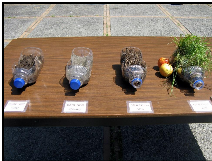
Figure 2. Four juice containers filled with a) bare soil (fine), b) bare soil (coarse), c) mulch on fine soil, and d) grass on fine soil.
